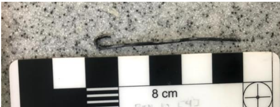
Figure 2: The wire of the historic repair of the ear flap after being removed. It was then cleaned using steel wool and 3-in-one oil, as was the hole it threaded through before being re-threaded and bent back into place, tighter than previously to support the hinge (photo by author)
